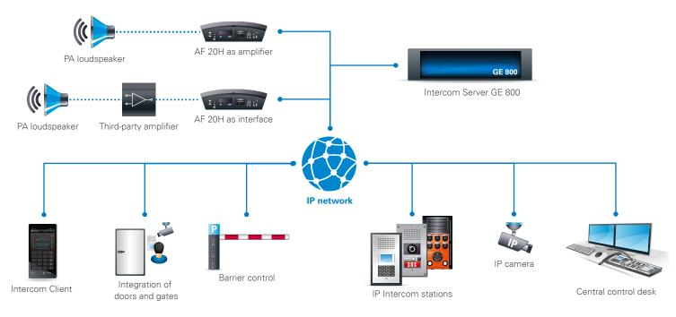
The following illustration shows an example of the integration of an AF 20H amplifier into an IP network.
